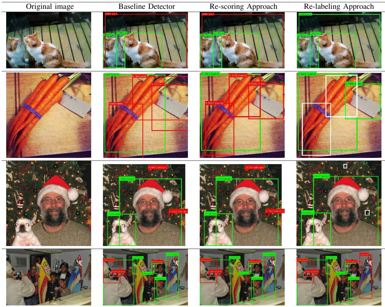
Fig. 14: Threshold 0.5: Relabeling and Re-scoring models outputs: Green, red and white boxes represent correct detection, incorrect detection, and objects removed and re-labelled as background, respectively
