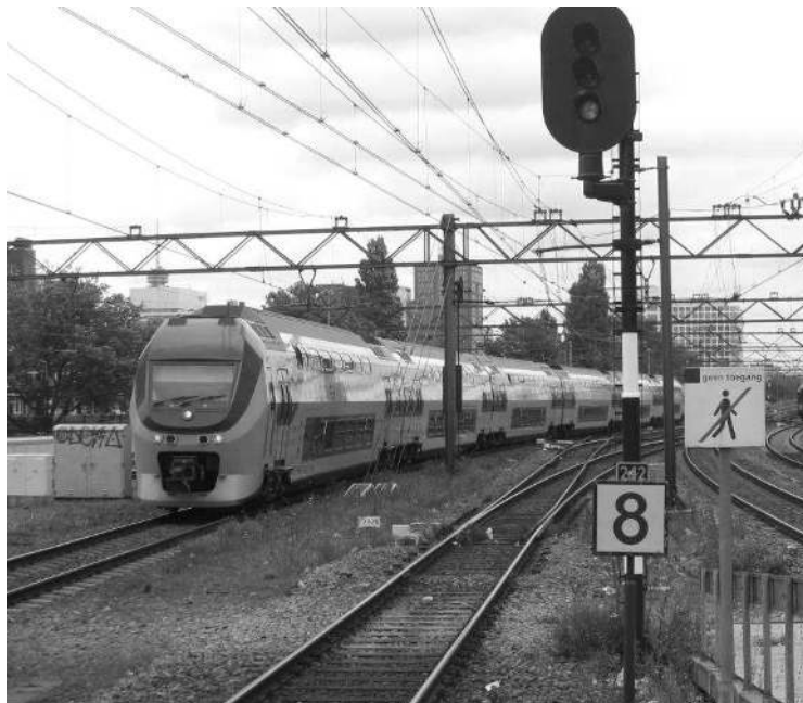
Figure 3.1: A train facing a red signal aspect while waiting for the passage of a preceding train
