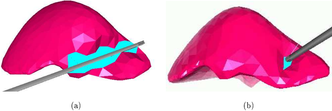
Figure 20: Modeling of contact between the surgical tool and the liver soft tissue model.
