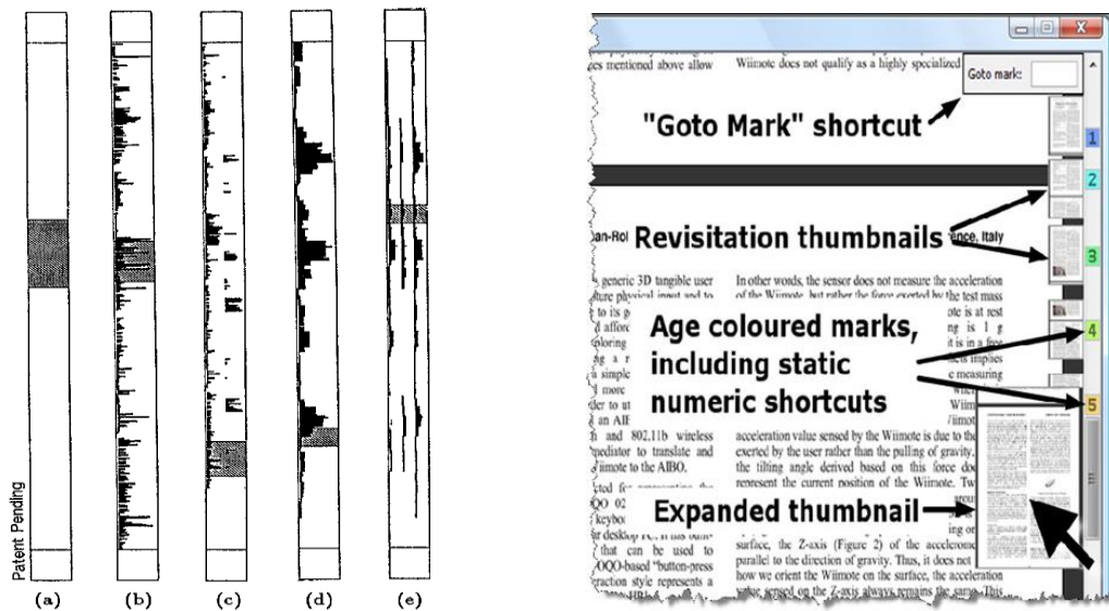
Figure 2.5. Implicit revisitation techniques. Left: Edit Wear and Read Wear (histograms in scrollbar show amount of user activity with that area of the document). Right: Footprints scrollbar, showing five previously-visited locations.
