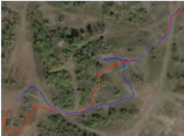
Figure 7. Comparison of paths executed by our robot for shown course when using only on-board perception (in solid red) and with OOLL (in dashed blue) and FROLL (in dotted cyan) used in real-time on-board the robot. Course started at the top right and ended at the bottom left.
