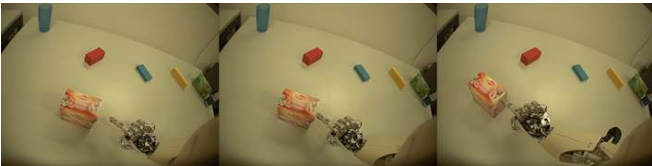
Fig. 4. An example of a series of images collected during a POKE action with the iCub robot.
