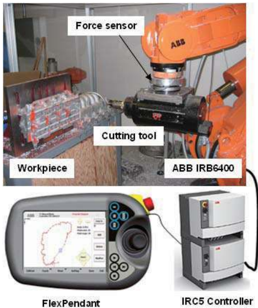
Fig.4 System Setup for Robotic Machining with Force Control (Note: This setup is using a development version of IRC5 controller. For the formal released IRC5, IRC6400 is replaced by a new IRB6640 robot.)
