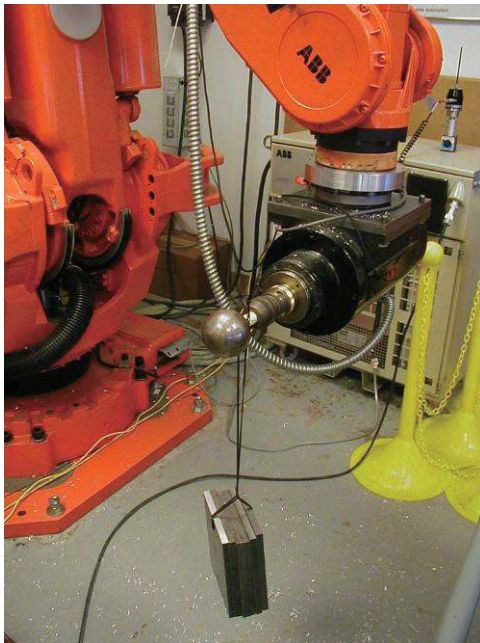
Fig.2 Methodology of robot stiffness measurement
