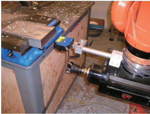
Fig.6 Setup of aluminum end milling and surface scan
