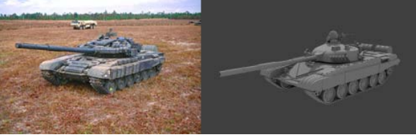
Fig. 3. MSTAR T-72 tank and T-72 CAD model used for simulated image.
