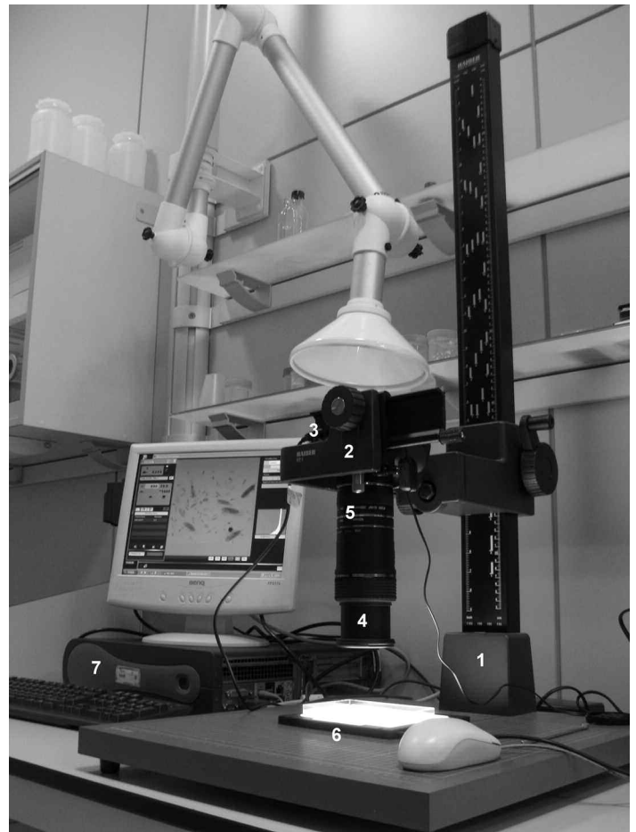
Fig. 2. Digital camera system: (1) Copy stand & tilting arm (model Kaiser RS1 5511); (2) Micrometric sliding plate (model Manfrotto 454); (3) Camera (model CANON EOS 450D); (4) Macro lens (model Tamron SP 90mm F/2.8 Di EOS); (5) Extension tubes (model KENKO 3 Ring DG P/Canon EOS, 12 + 20 + 36mm); (6) Uniform white LED backlight (model BIBL-w130/110); (7) Connected computer system.
