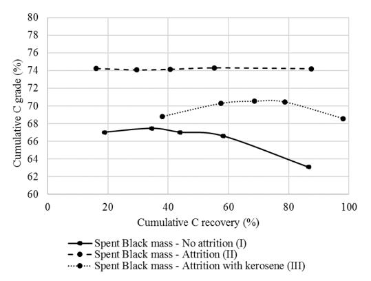
**Figure 3.** Grade and recovery of carbon in the overflow product according to the flotation flow: no attrition (II), with attrition (II), and attrition with kerosene (III).
