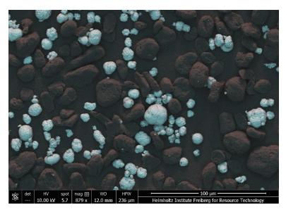
**Figure 5.** SEM image with imposed colors of the model black mass before attrition. LMO particles in blue and graphite particles in black.
