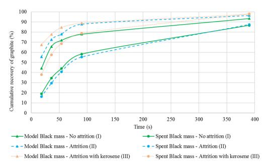
**Figure 9.** Carbon recovery from the spent black mass and model black mass in the overflow product according to the flotation time.
