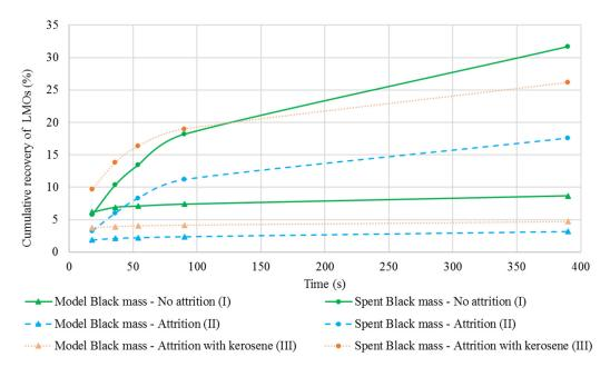
**Figure 8.** Recovery of the LMOs from spent black mass and model black mass in the overflow product according to the flotation time.
