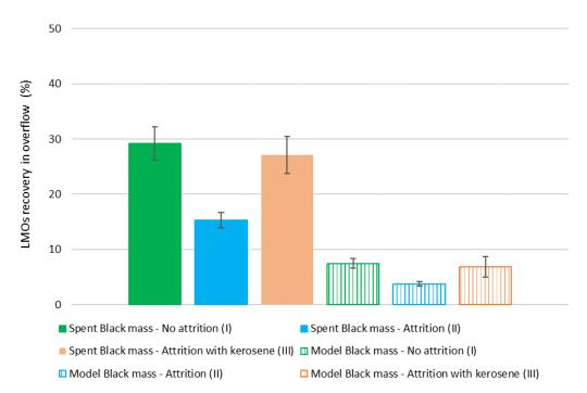
**Figure 7.** Recoveries of LMOs (including Co, Ni, and Mn elements) from spent black mass and model black mass with the different flotation flows: no attrition pre-treatment, with attrition pre-treatment, and attrition pre-treatment with kerosene. The results are average values of four experiments and the error bars represent an interval confidence of 90%.
