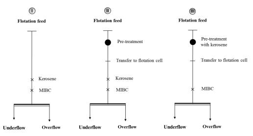
**Figure 2.** The three flow diagrams for the flotation experiments. (I) No pre-treatment, (II) With pre-treatment, (III) Kerosene added during the pre-treatment.
