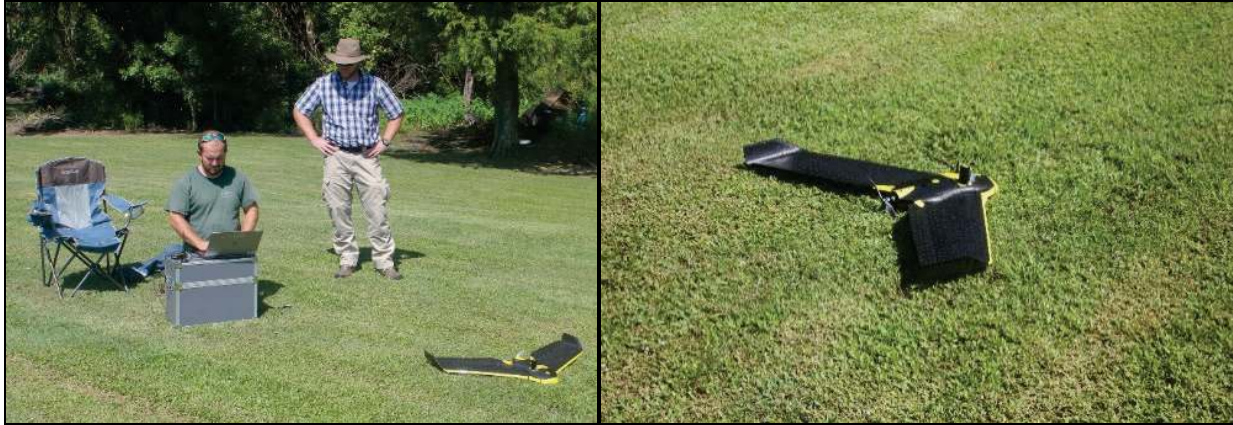
Figure 2. Fixed-wing senseFly eBeeRTK used to acquire aerial images.
