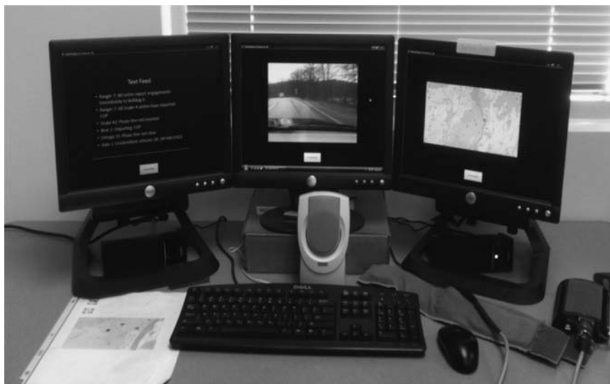
Figure 1. Experimental task and environment. Shown are three monitors, each with a speaker mounted below, keyboard and mouse. Also shown are the factor belt with battery pack and reference sheet illustrating visual targets that appear on screens two (route markers) and three (blue force tracker symbols) (Colour online).
