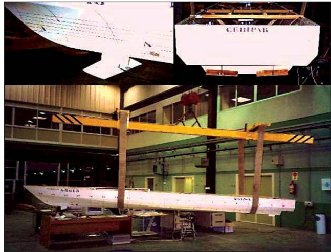
Figure 16. The scale model out of the water. At bottom, the scale model is hanging from a fulcrum attached to a crane, which allows verification of actuator motion. Top left is a view of the T-foil, while top right is the transom flaps. The actuators are moved by electric motors.
