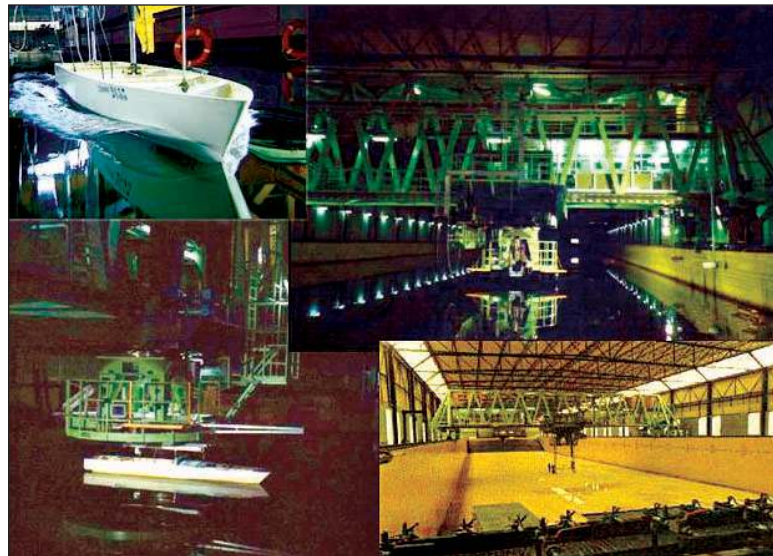
Figure 6. Experimental devices and facility. Top left is the scaled-down replica on calm waters. Top right is a view of the 150 m \times 30 m basin with the wavemaker and computerized planar motion carriage. Bottom left is a detail of how the replica (4 m long) is attached to the carriage. Bottom right shows a view of the empty basin with people inside.
