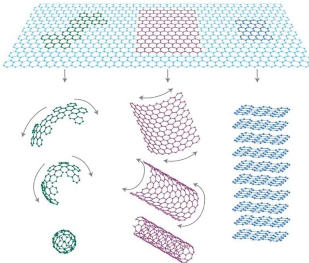
**Fig. 8** Graphene in various forms; it can be wrapped up into 0D buckyballs, rolled into 1D nanotubes or stacked into 3D graphite.<sup>134</sup> Reprinted with permission from ref. 134 (Copyright © 2007 Nature).
