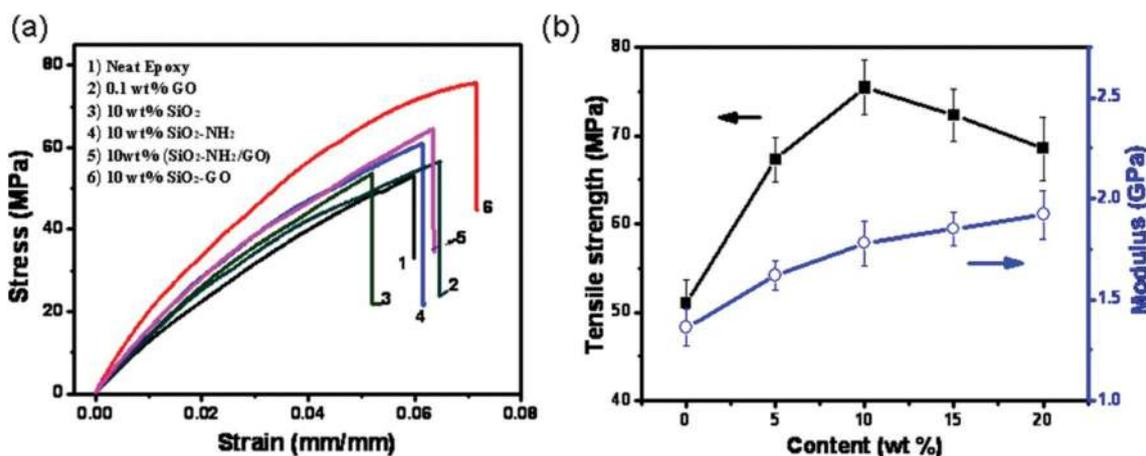
Fig. 14 (a) Stress-strain curves for neat epoxy and epoxy composites; (b) effect of SiO<sub>2</sub>-GO content on the tensile strength and modulus of epoxy resins.<sup>196</sup> Reprinted with permission from ref. 196 (Copyright © 2012 ACS Publication).
