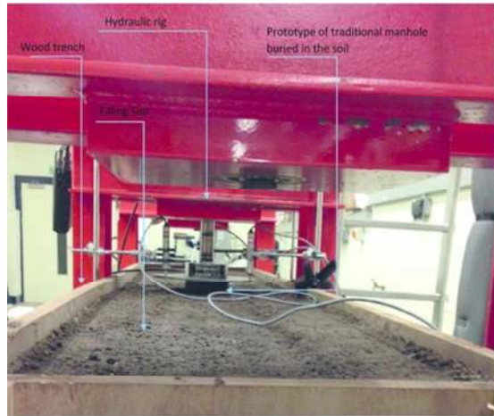
Fig. 7 a. Setup of the trench in the rig and location of measurement instruments on the traditional manhole surface at three points on the edge.
