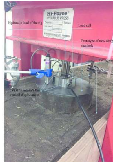
Fig. 6 b. Setup of the trench in the rig and location of measurement instruments on the new manhole surface at three points on the edge.
