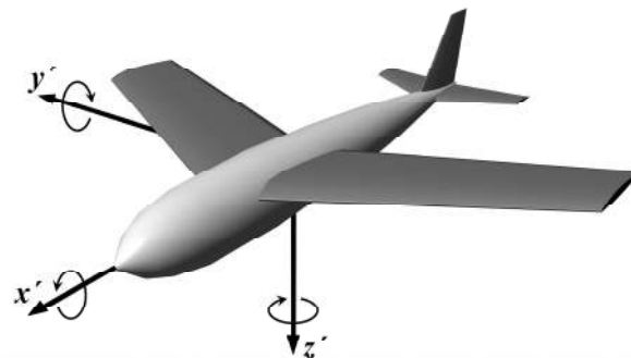
Figure 1. Orientation of the coordinate system axes.
