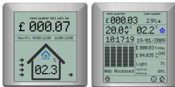
Figure 3.1: Virtual control panel of domestic central heating
