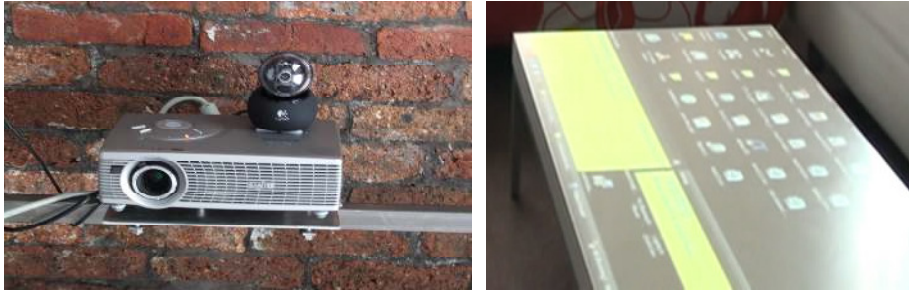
Figure 5.2: The projector (left) rendered interfaces on the coffee table (right)
