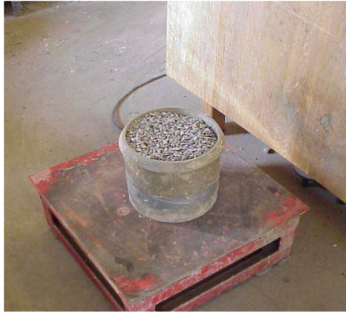
Figure 11 Steel bucket placed on vibrating table
