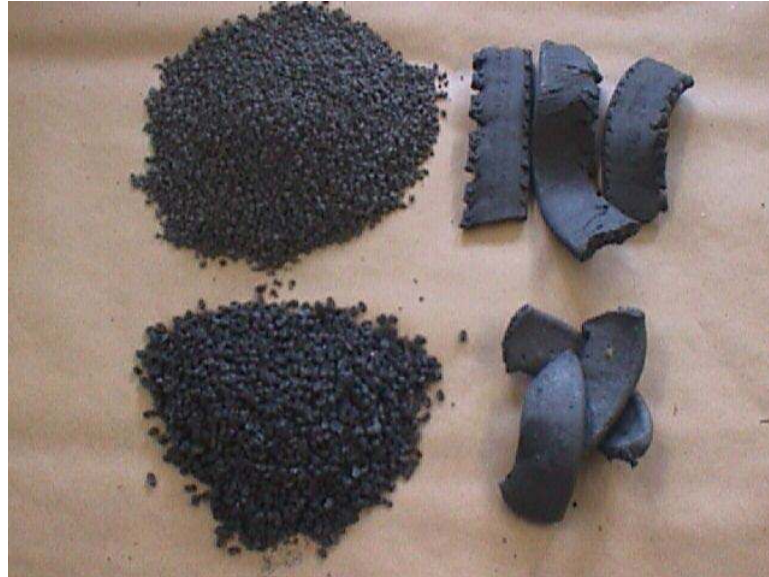
Figure 8 Synthetic Lightweight Aggregate strips and granulated
