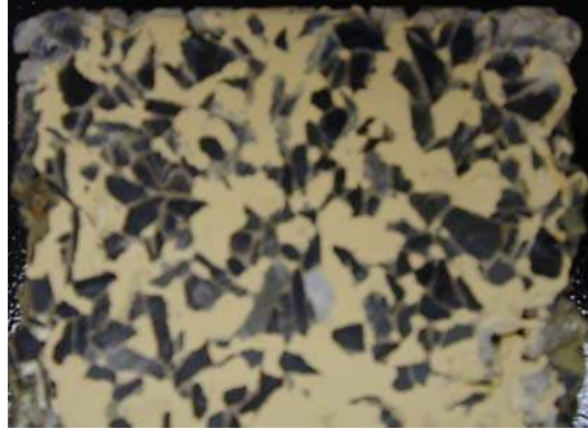
Figure 17 Concrete pores filled with Wood Putty®
