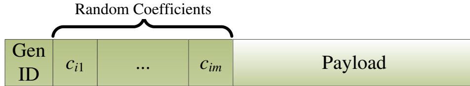
Figure 2.7 Network Coding packet format
