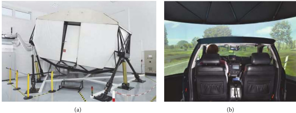
FIGURE 1: The WIVW dynamic driving simulator. Hexapod movement system (a) and simulator interior with vehicle mock-up and video projection (b).
