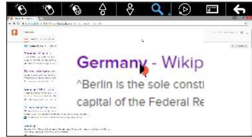
(b) Magnified screen as second step in mouse click emulation for more accurate pointing.
