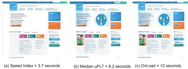
Figure 1: Snapshots of the page load of energystar.gov shown at the Speed Index, the median uPLT across 100 users, and OnLoad values.
