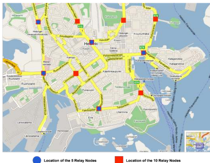
Fig. 2. Helsinki simulation area with the locations of the relay nodes.
