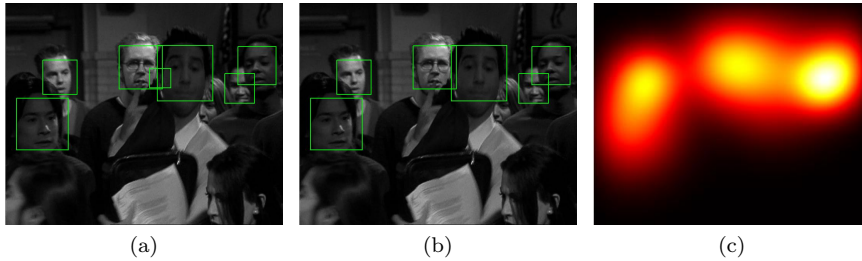
Fig. 3: Raw face detections (left), post-processed face detections (middle), face saliency map M_f after post-processing (right)
