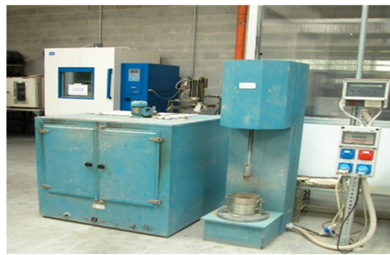
Figure 5. Determination of OMC and MDD with a proctor test.
