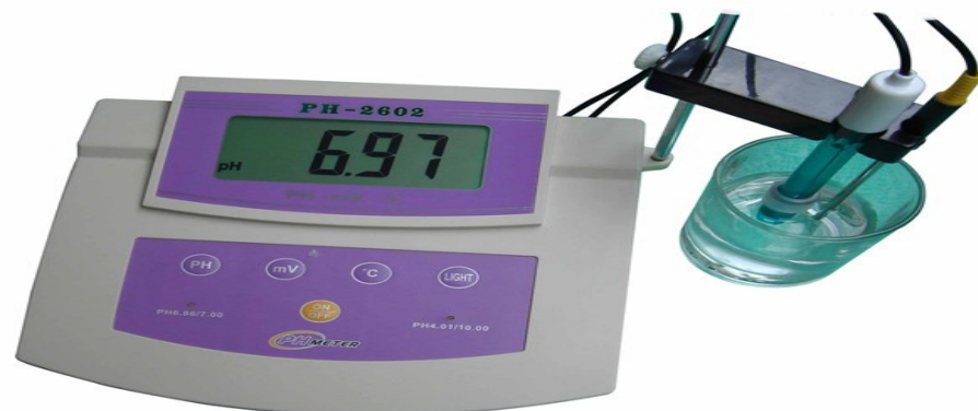
Figure 6. Determination of pH of samples with pH meter.
