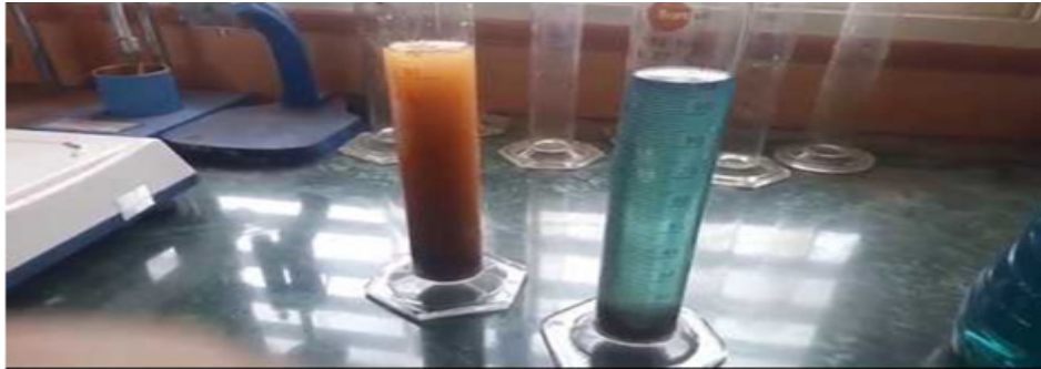
Figure 1. Free swelling test apparatus.
