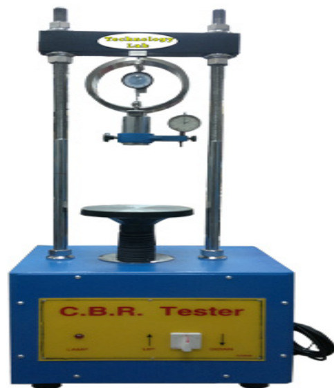
Figure 4. Determination of CBR with a CBR apparatus.
