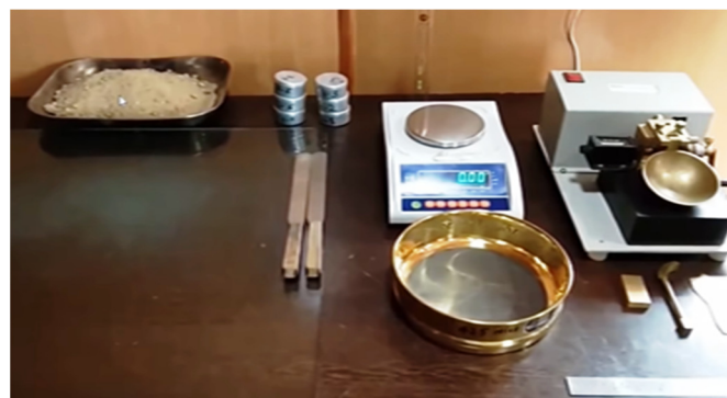
Figure 3. Determination of LL and PL with a Casagrande apparatus.
