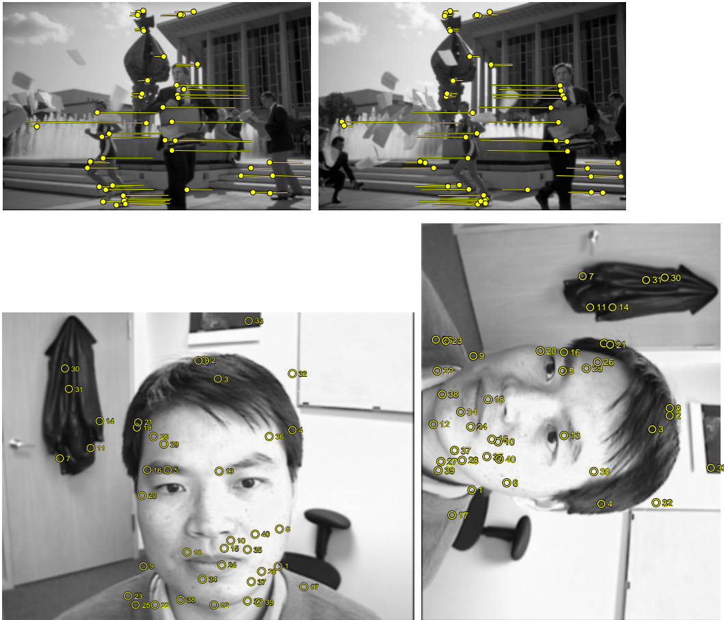
Figure 2: Top Row Wide Baseline Success of IMPSAC: the first and last images from the Samsung sequence, captured at the same time but from different positions. The disparity between the images is up to 160 pixels, yet only 3 or 4 of the 50 example matches shown are mismatched. Bottom Row Rotation Success of IMPSAC: Despite the combination of a rotation of 90 degrees and the change in pose of the face, the features are correctly matched. Although just 40 features are shown for clarity, over 1000 were matched.
