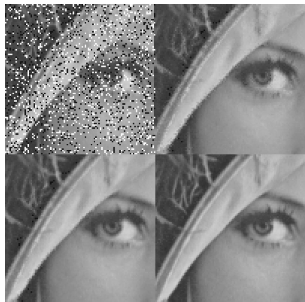
Fig. 5 (a) Enlarged area of ‘‘Lena’’ corrupted by 20% fixed-valued impulse noise, (b) restoration result by the one-order PA filter, (c) restoration result by the AOPA filter, and (d) the original image area.
