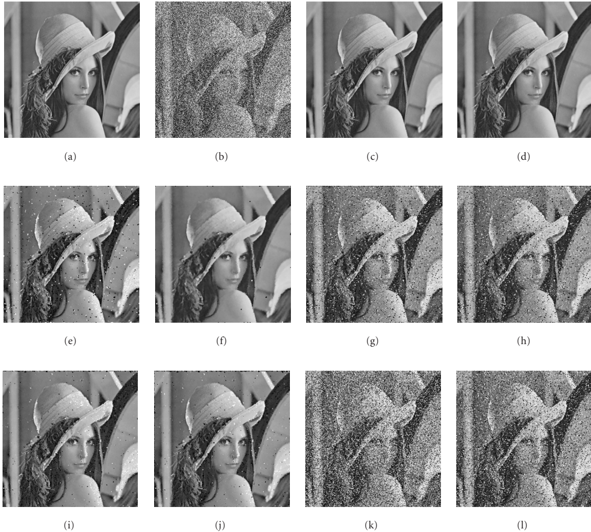
FIGURE 2: Restoration results of the Lena image for the noise density of 50%: (a) original Lena image, (b) corrupted Lena image (noise density = 50%), (c) NEF (proposed), (d) MMEM, (e) PSM, (f) IMF, (g) IRF, (h) SMF, (i) AMF, (j) SDR, (k) MSM, and (l) TSM.
