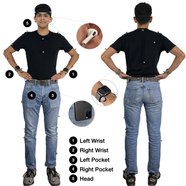
Figure 5: IMUPoser data collection setup. Participants wore 2 smartwatches, kept 2 smartphones in their front pockets, and wore wireless earbuds. 41 retroreflective motion capture markers were also placed around the body to track ground truth body pose.
