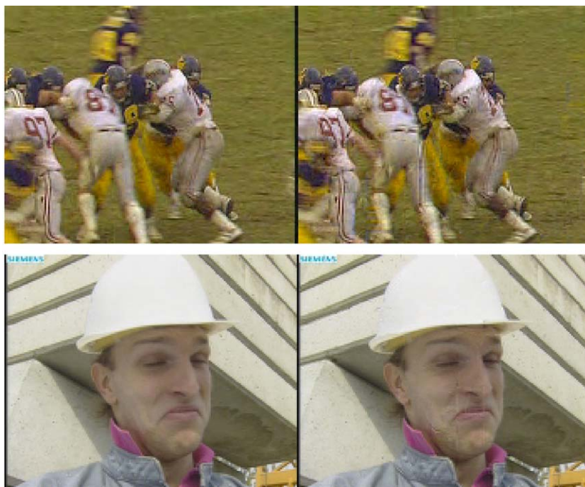
Fig 11. Visual comparison for the half-resolution/half frame-rate decoding at 768 kbps with IBMCTF (left) and SDMCTF (right). Even at high bit-rate, due to the fact that spatial filtering and motion compensation are not commutative in SDMCTF [3], motion artifacts are occasionally observed in the areas with irregular motion (player leg in the middle area of football, mouth of foreman).
