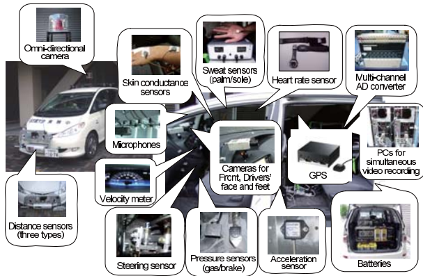
Figure 2: Sensors mounted on vehicle
