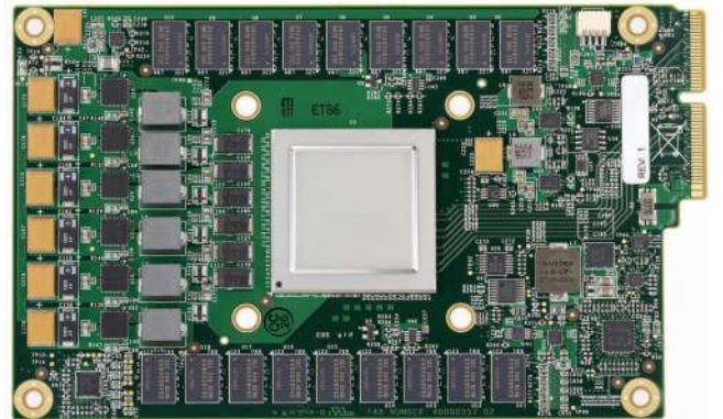
Figure 3. TPU Printed Circuit Board. It can be inserted into the slot for a SATA disk in a server.
