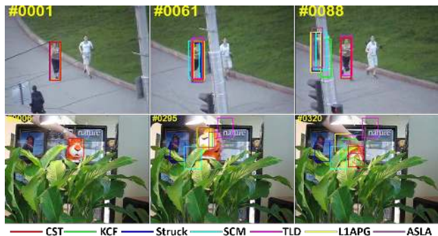
Figure 1. Comparison of our CST tracker with state-of-the-art methods (KCF, Struck, SCM, ASLA, L1APG, and TLD) on two videos from a visual tracking benchmark [32]. On the Jogging sequence, only TLD and CST can track well when partial occlusion happens. On the Tiger sequence, our CST can track the target throughout the whole sequence, while other trackers suffer from drift. The sparse trackers (ASLA, L1APG, SCM) fail to track these sequences. Overall, the proposed CST method performs favorably against the state-of-the-art trackers.
