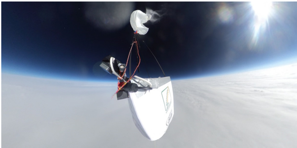
Figure 21. The view from the 360° camera affixed on the main gondola's lid at the moment of the balloon burst at the maximum reached altitude. Below the gondola, the upper surface of the encountered storm front can be seen. The visibility inside the storm front dropped to single meters.
