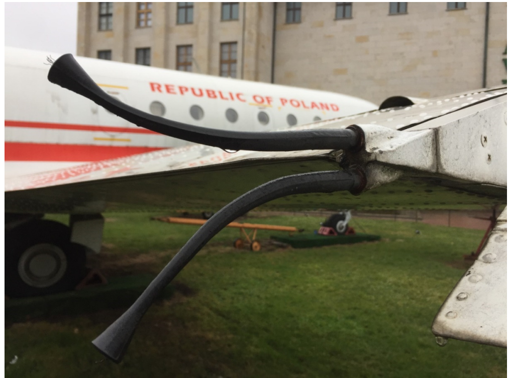
Figure 1. Electrostatic dischargers permanently riveted onto the rear part of the wing of the Yakovlev Yak-40 no. 044 (Polish Air Force); the rubber insulation, expanding at the end, moves away from the corona-susceptible wire bundles from the aircraft's structure; the wire bundles are easily noticeable at the ends of the cables. The airplane has such dischargers affixed on both wings and on the upper part of the vertical stabilizer.
