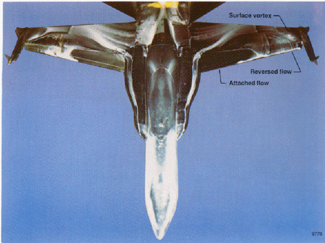
(c) Oil flow visualization of surface streamlines, 0.06-scale model of F-18 HARV, Langley Research Center 14- by 22-Foot Subsonic Tunnel, \alpha = 25^\circ .
