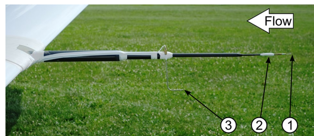
Fig. 1 Boom with (1) x-wires, (2) accelerometers and (3) Prandtl-tube attached to sailplane wing nose
