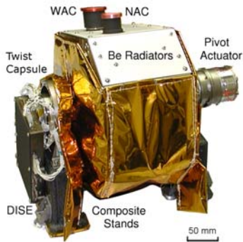
Fig. 1. The fully assembled MDIS instrument showing key components. All electrical connections pass through a rigid-flex assembly rotary interface (twist capsule).
