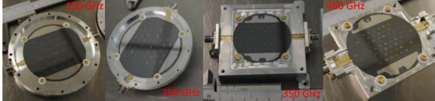
Fig. 2 Pictures of the four OLIMPO detector arrays mounted in their ergal (aluminum 7075) holders by means of four Teflon washers 100\ \mu\text{m} thick. From left to right : the 150 GHz, 250 GHz, 350 GHz, and 460 GHz arrays.
