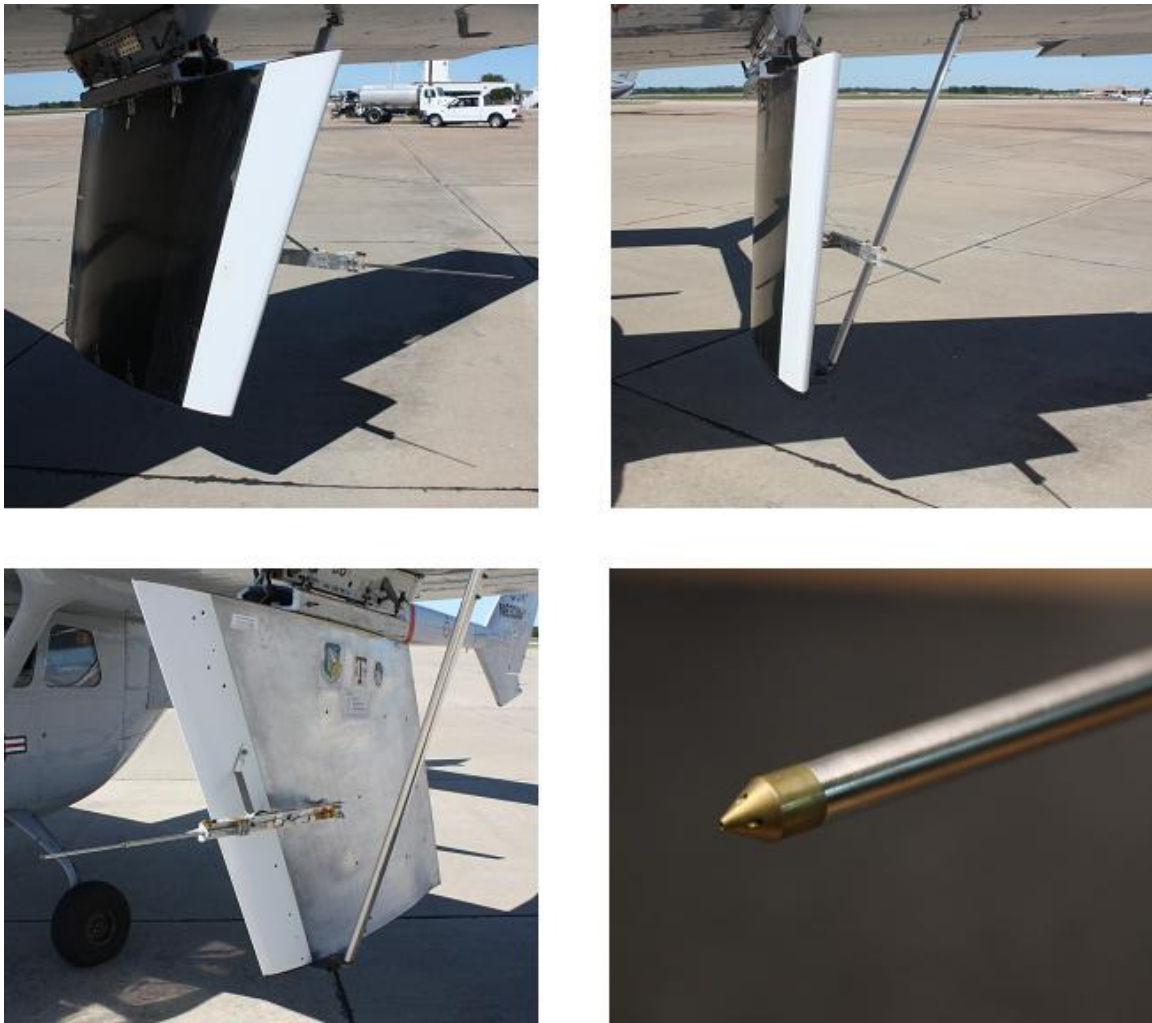
Figure 10: Five-hole probe mounted to SWIFT model.
