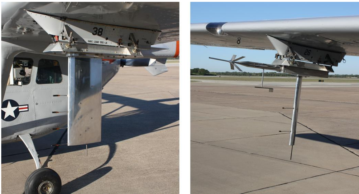
Figure 13: Hotwire sting mounted to the port outboard pylon and air data boom mounted to the starboard outboard pylon.
