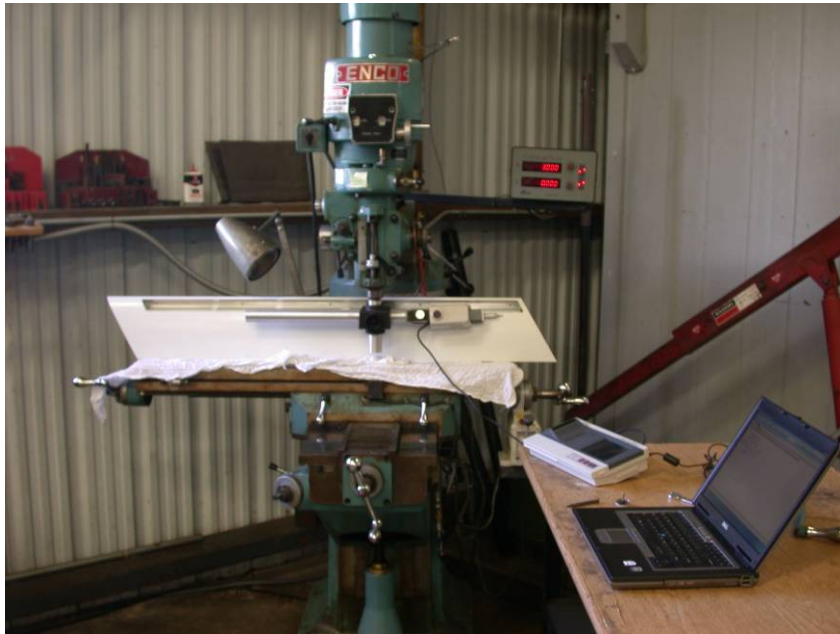
Figure 12: Picture of surface roughness measurements on the SWIFT leading edge.
