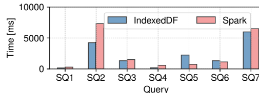
Fig. 13. The improvement of the SNB queries on Indexed DataFrame versus Spark on an input dataset of SF 300.
