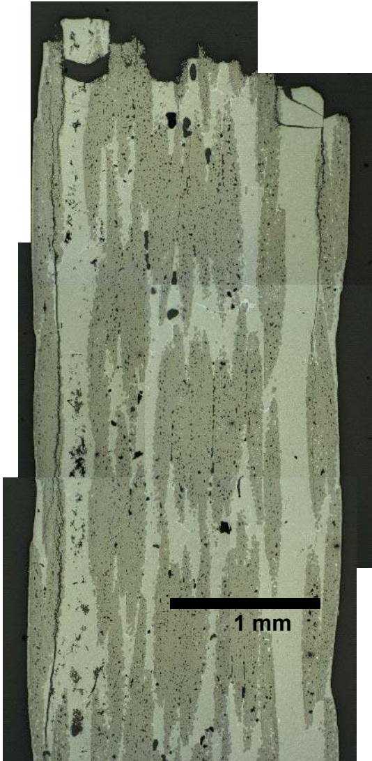
Figure 8: Micrograph of a 2D woven 45/45 oriented composite after RT tensile failure.
