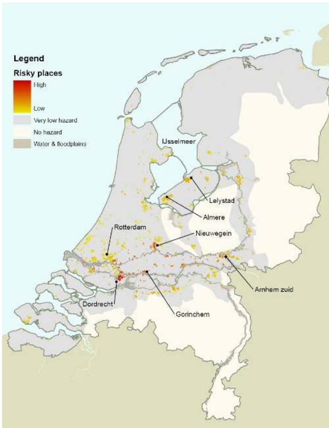
Fig. 3. At “risky places” unbreachable embankments may be very effective in reducing the risk of loss of life (De Bruijn and Klijn, 2009).
