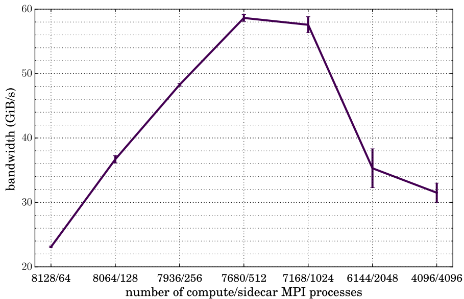
Figure 6 Total bandwidth during transfer of a 10-component 1,024 3 grid (32,768 Boxes) among 8,192 total MPI processes, with varying sizes of compute and analysis groups. The standard deviation over 5 iterations is indicated with error bars.
