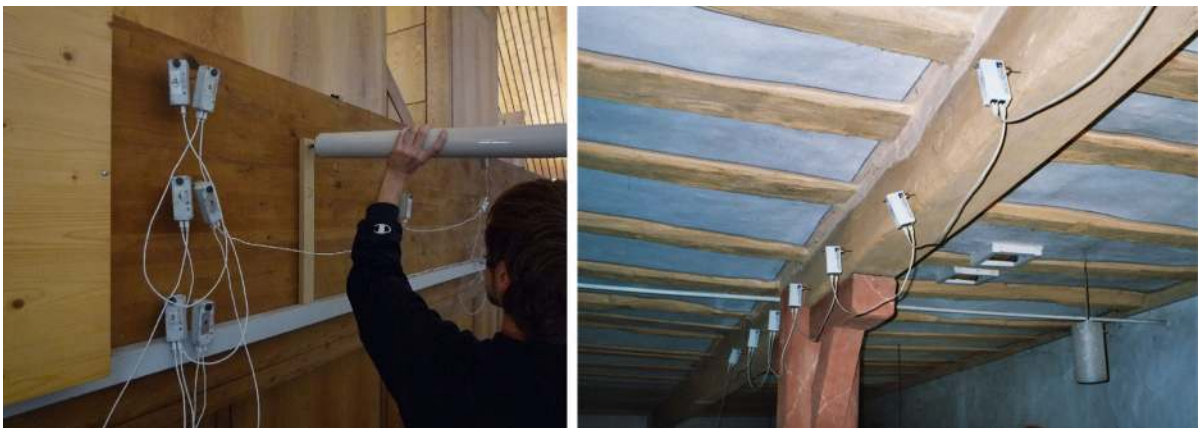
Fig. 8 Typical examples of TOF measurements: on glulam beams ( left ) and ceilings ( right )
