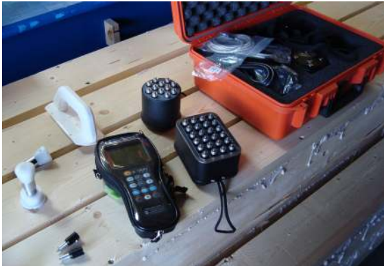
Fig. 12 Sensor head for ultrasonic echo technique
