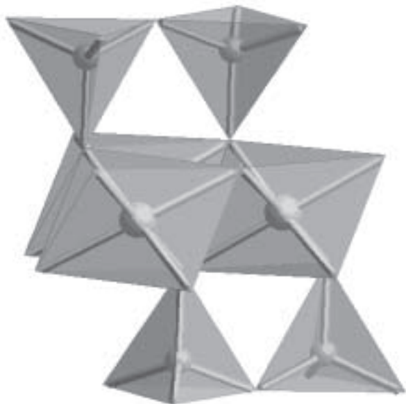
FIGURE 9. One stoichiometric crystal growth unit for a trioctahedral 2:1 phyllosilicate, assuming random substitutions.
