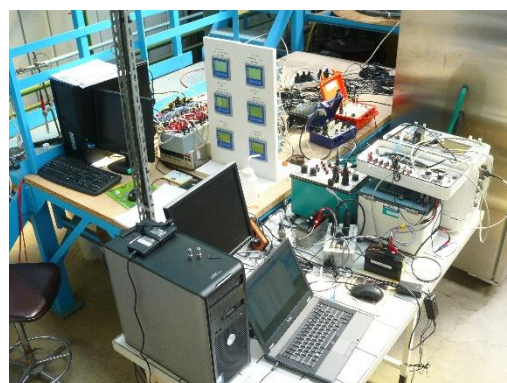
Figure 6.7. Setup and apparatuses for the monitoring of the physical and chemical parameters of the column output water and geophysical electrical measurements into the column (and over the length of the column).
