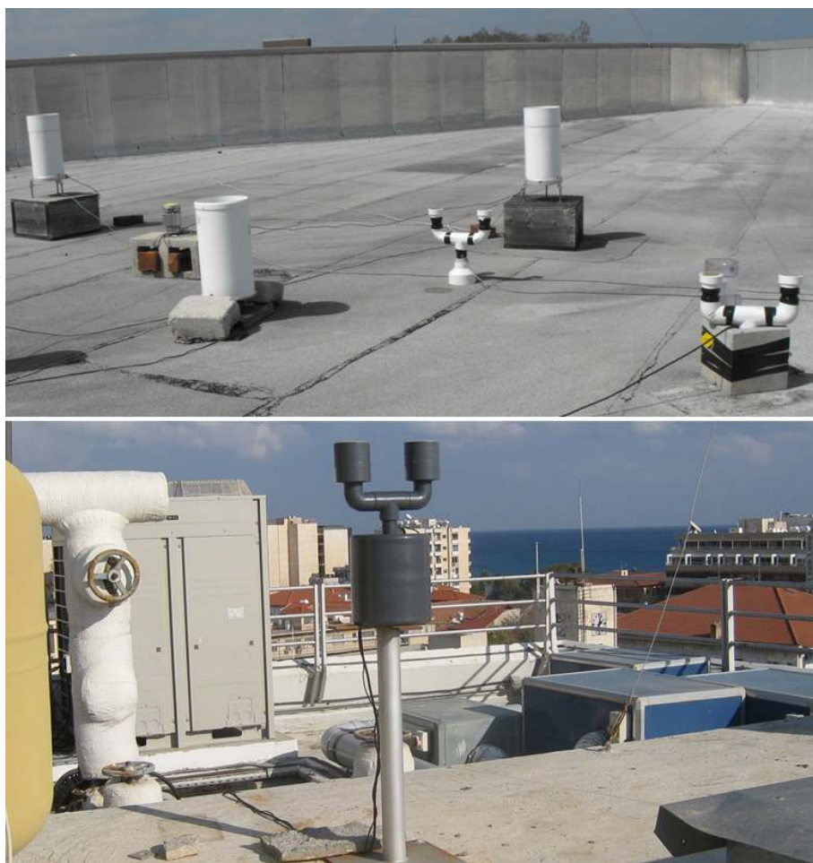
Fig. 16. Roof of UCF Engineering Building, showing three tipping bucket rain gauges (white cylinders) and three disdrometers: Joss disdrometer on the left, and two UCF-DHD disdrometers in the center and far right (top), and CUT-DHD on the roof of the Cyprus University of Technology (bottom).
