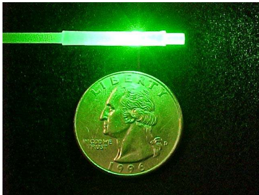
Figure 13. Stimulated Sensor Showing Light Scatter at the Fiber/Fiber Optic Interface
