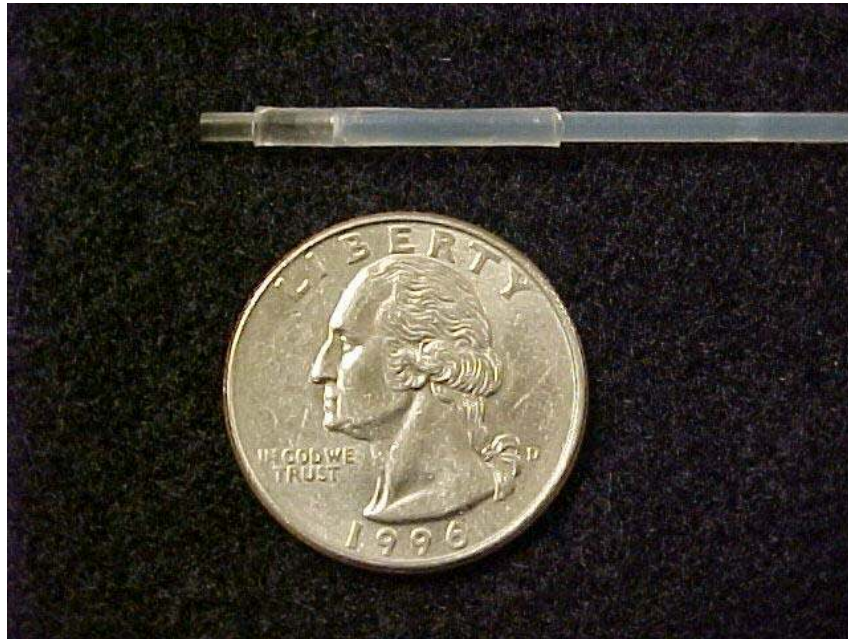
Figure 12. Unlighted Sensor Showing Interface between the \text{Al}_2\text{O}_3 Fiber and the Silica Fiber Optic Channel
