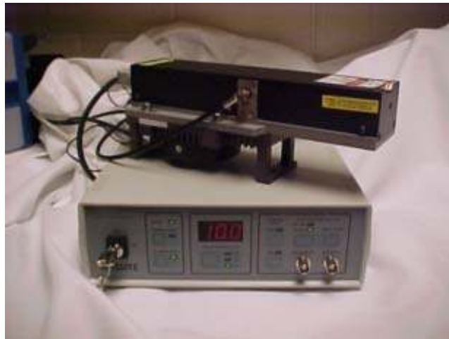
Figure 21. Pulsed Laser and Power Supply to be Incorporated into a Portable Reader
