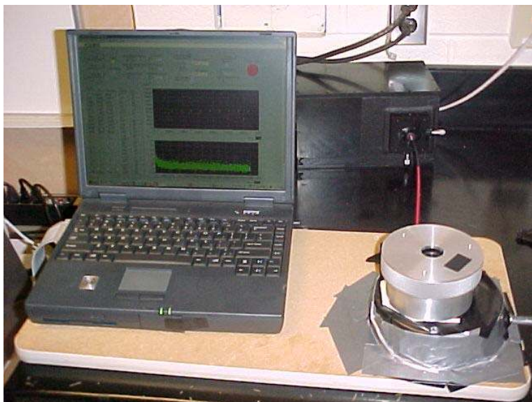
Figure 10. The OSL Reader System, Including the Reader (Background), the Red Fiber Optic Channel, the Irradiation/Readout Chamber, and a Laptop Computer for Data Acquisition
