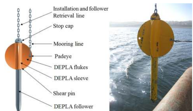
FIG. 3 Dynamically embedded plate anchor.
