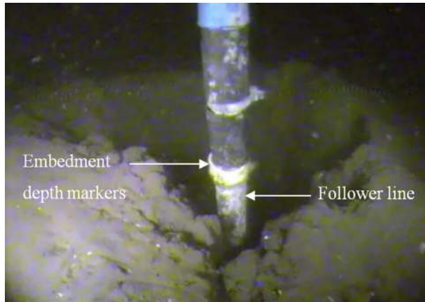
FIG. 12 Image capture from ROV camera showing the follower retrieval line at the seabed.
