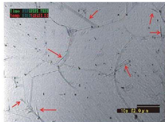
Fig. 11 Nucleation of bainitic ferrite in Fe-0.15%C steel.
